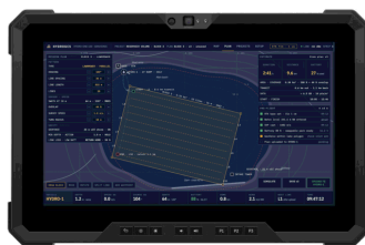
Plan · Survey lines, estimated time and pre-survey checks
